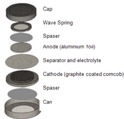
Figure 1. Design of aluminum ion battery (coin cell).
