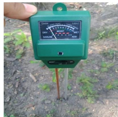
Gambar IV. Mengukur pH tanah Plot I
