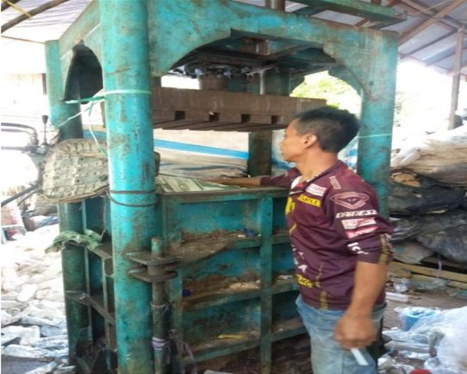
A man in a maroon shirt is operating a large, blue industrial press machine. The machine is used to compress plastic waste into bales. The setting appears to be an outdoor or semi-outdoor industrial facility.                                                                 |
